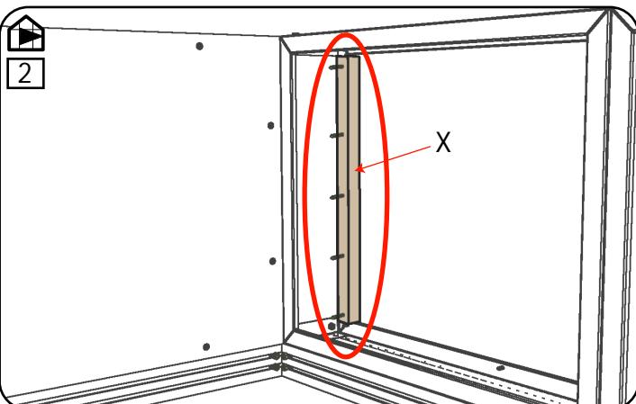
Fiber cement plader - Fibre cement sheeting - Faserzementplatten - Fiber cement platter
