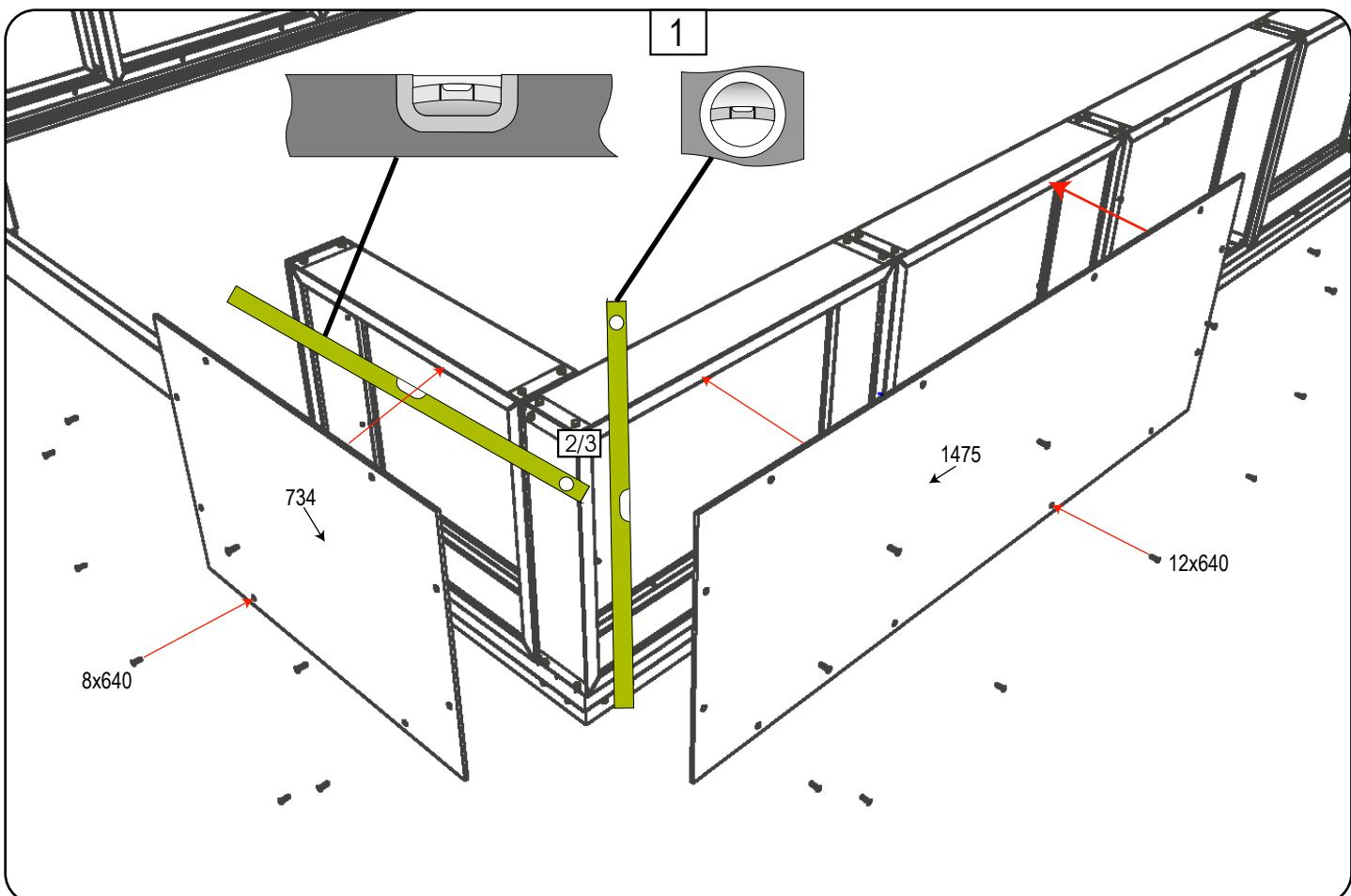
**Fiber cement plader - Fibre cement sheeting - Faserzementplatten - Fiber cement platter
