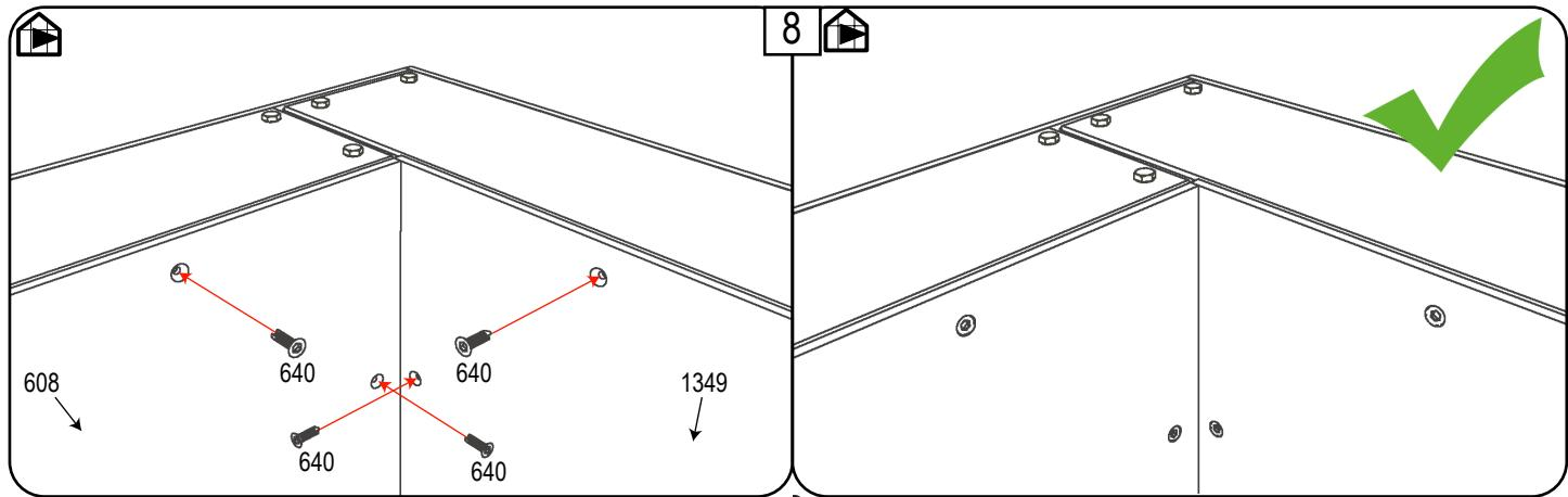
Fibercementplader - Fibre cement sheeting - Faserzementplatten - Fibercementplattor
